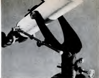
ALTAZIMUTH MOUNT provides independent motion in both vertical and horizontal planes. But it must be moved in both directions at once to follow the path of a star as the earth rotates.
